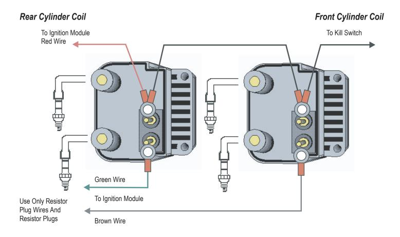
IMPORTANT NOTE: DF coils can not be wired for 2 plug per cylinder Dual Fire. You are jumping double the gap under compression when dual plugging. If both plug on same cylinder are gapped at 0.040" your jumping 0.080 under pressure. Would you gap a single plug at 0.080 under raised compression. Recommended sparkplug gap setting no more than 0.025"
